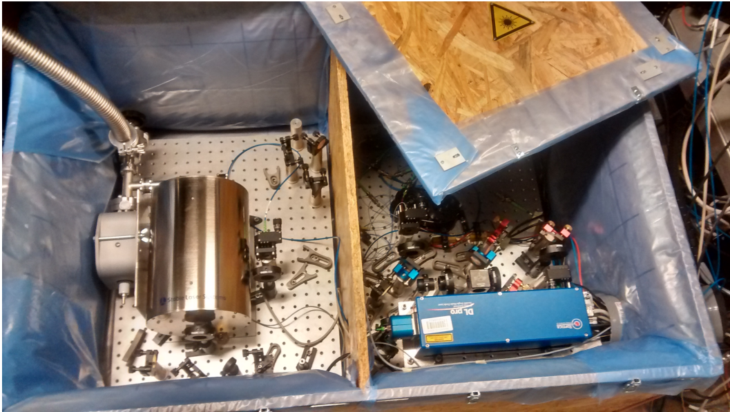
Figure 5.2: Custom isolation box for two 1160 nm laser sources (stacked vertically on the right of the picture) and the high finesse optical cavity used for frequency stabilization (inside a vacuum chamber, on the left). Of the two lasers, only the one below, not visible here, is used in the experiments described in this thesis. This arrangement allows to spatially decouple the sources from the rest of the setup, connected via optical fibers, and improve thermal and acoustic stability. As a results, the frequency lock could operate continuously without human intervention for multiple consecutive months.
