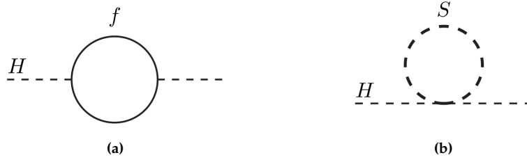
Figure 1.4 – One-loop quantum corrections to the Higgs squared mass parameter m_H^2 , due to a Dirac fermion f (left), and a scalar S (right) [24].
