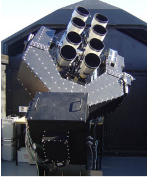
Figure 4.1 : The eight SuperWASP cameras are installed together on one equatorial mount. Image credit D.R.Anderson.
