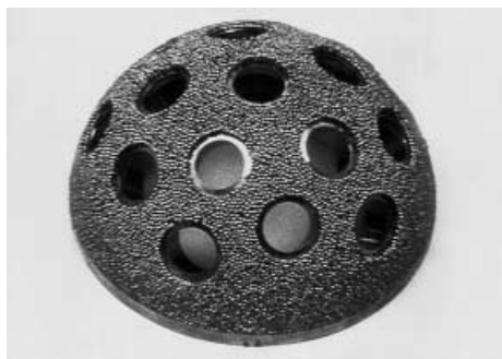
Fig. 1 Opti-Fix cup . Porous coating with titanium beads. Holes allow additional screw fixation at multiple sites
