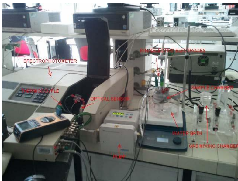
Scheme S8.1. Representation of the experimental apparatus. The sample compartment is placed in a thermostated water bath (not shown). A photograph of the setup is shown below.
