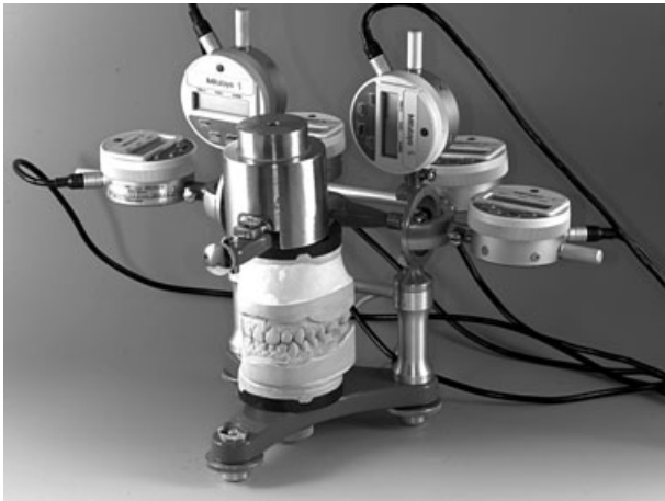
Fig. 1. Measuring device with relocatable load of 10 N on the upper part which records the habitual occlusion in the condylar area in three dimensions.
