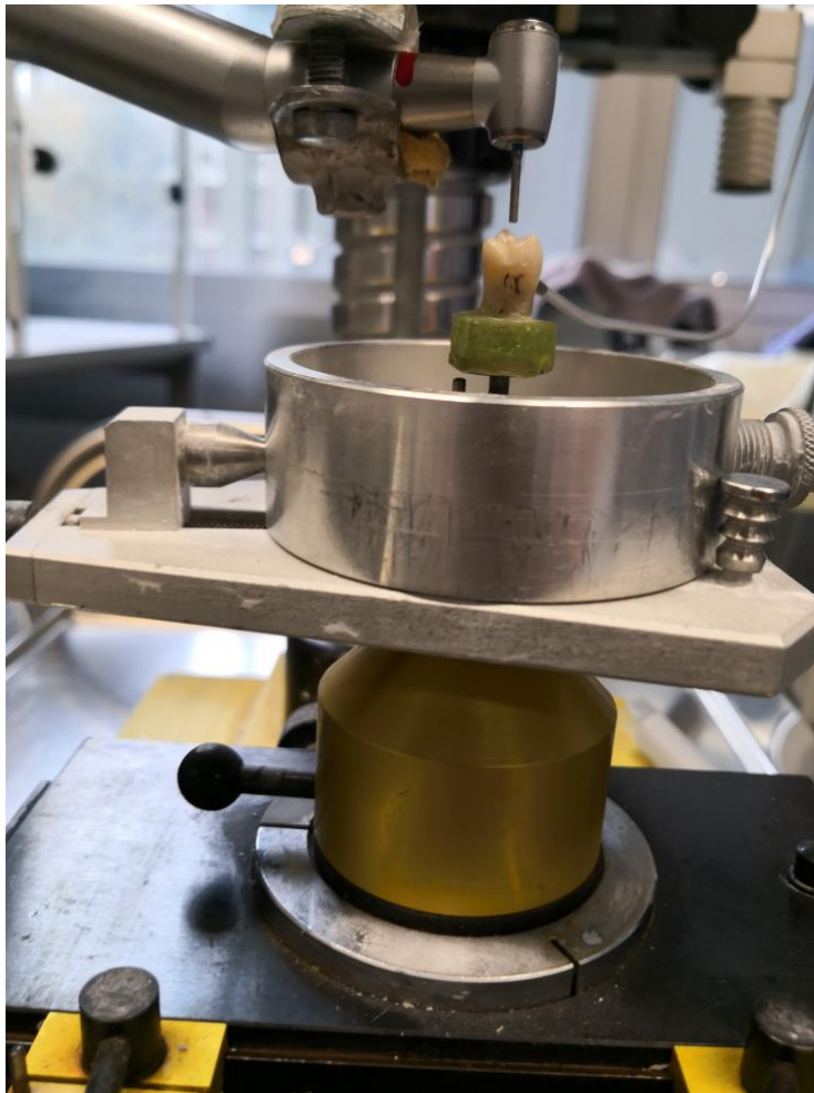
FIGURE 3: Photograph of the handpiece holder that allows to perform standardized cavities by restricting the bur's position.
