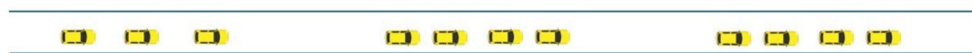
Fig. 2 Three platoons, the leader of each platoon can accelerate since the head-tail distance with the last trailing car of the next platoon is large enough, i.e. its speed is free
