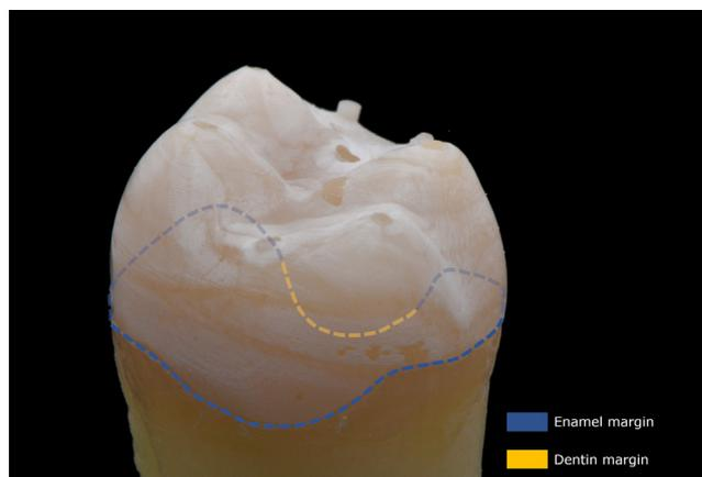
**Figure 1.** Three-dimensionally printed composite resin specimen before finishing and polishing along cavity outline with margins in enamel and dentin.
