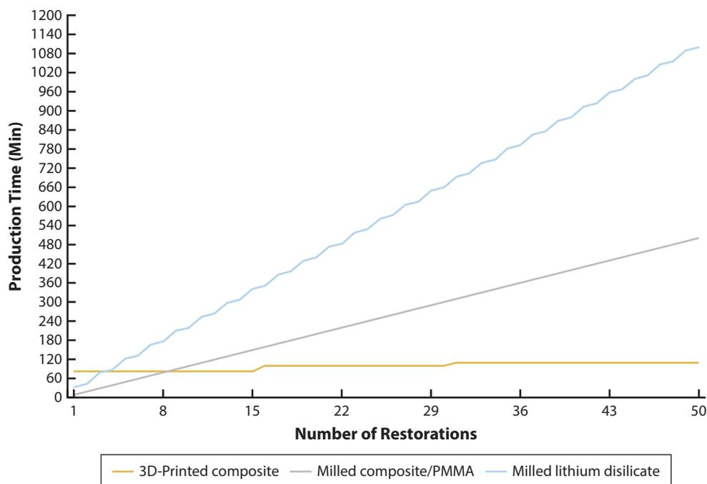
**Figure 4.** Time of production in minutes of all tested materials in function of number of restorations.
