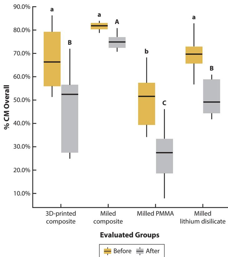
**Figure 3.** Box plot of continuous margin (%CM) percentages before and after fatigue for all evaluated groups. Different lowercase letters indicate groups with statistically significant difference before fatigue, and different uppercase letters indicate groups with statistically significant difference after fatigue according to Fisher LSD post hoc test. PMMA, polymethyl methacrylate.
