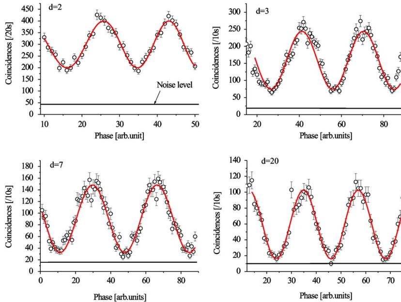
FIG. 2. Two-photon interference visibility for different dimensions  $d$ . The solid line is a sinusoidal fit from which we can deduce the net visibility of the fringes. The level of accidental coincidence is indicated by the straight line.
