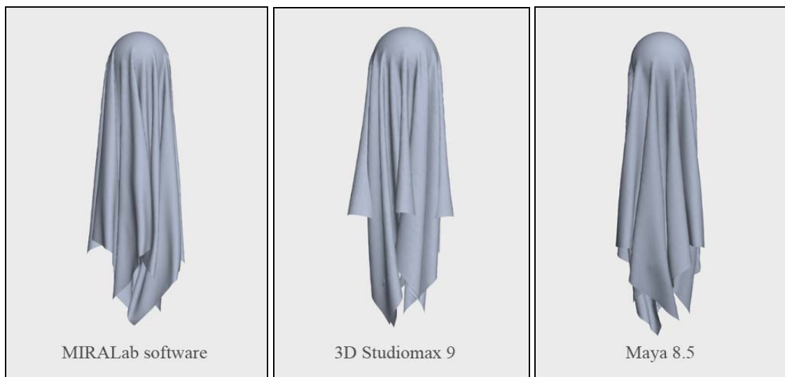
Figure 57: Simulated cotton fabric with MIRALab's in-house simulation application, Figure 58: 3ds max 9 (ClothFX) simulation application, Figure 59: Maya 8.5 (MayaCloth)
