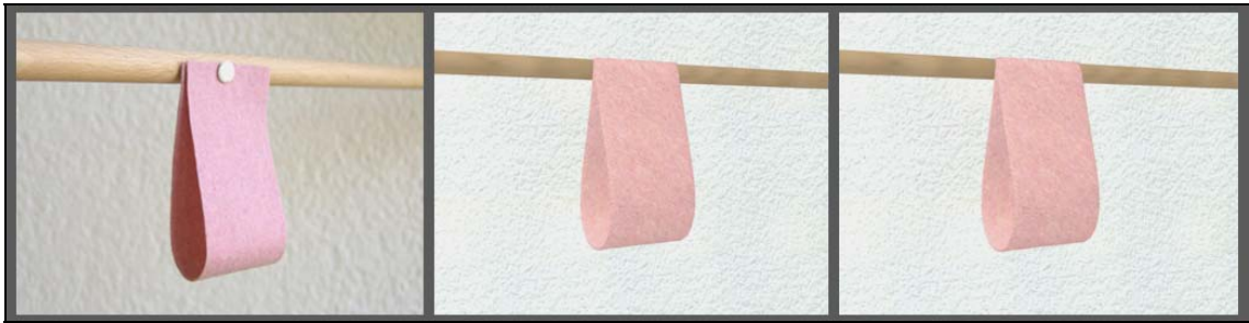
Figure 93: Real bending loop front, KES-f bending loop, FAST bending loop
