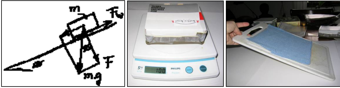
Figure 154: Scheme of friction evaluation [Tribol]
