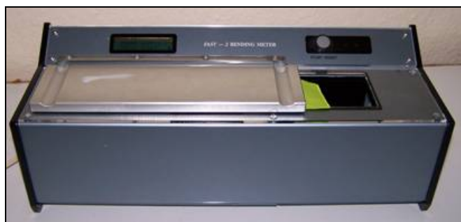
Figure 16: SiroFAST bending measurement machine [CSIRO 07]
