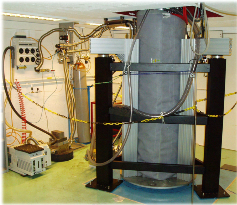
Figure 2.8: Aurora cryostat, low-noise nylon pumping lines and anti-vibration system.
