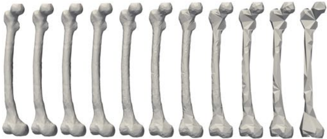
Figure 6.18 – The effect of the decimation on the model of the femur. The original model (left) is reduced to fewer vertices while preserving shape features like the femoral head and the condyles.
