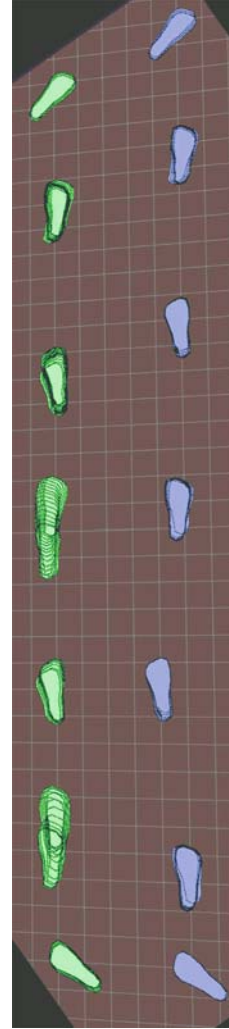
Fig. 4. Two foot prints left by a character animation: on the left (in green) the original clip and on the right (in blue) the retargeted clip. The residual sliding that one may notice in the blue prints is due to the estimation of the root motion between two steps, which makes both feet move at the same time in order to get a more realistic final motion
