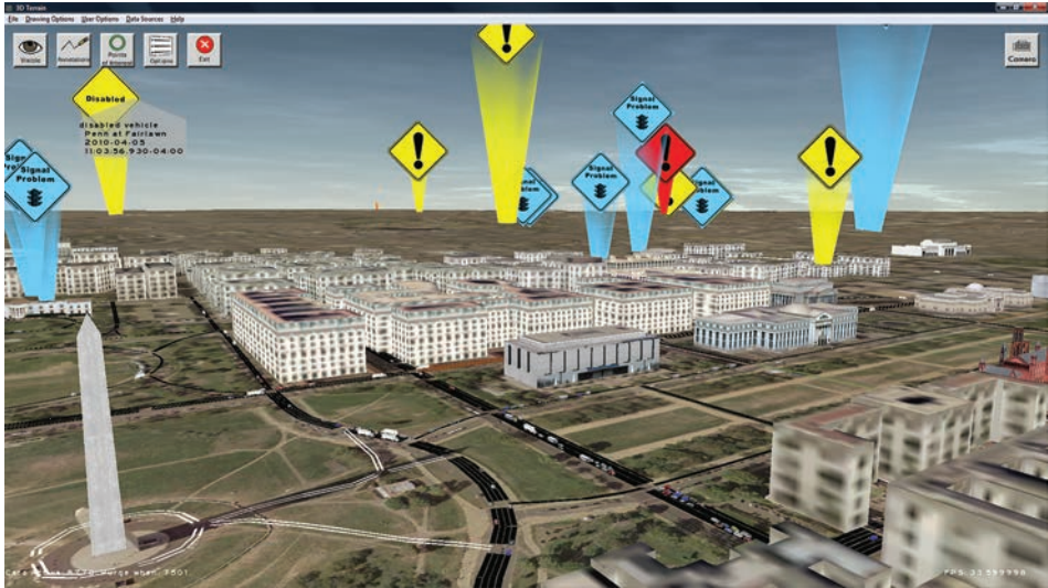
Fig. 8. Screenshot of a 4D real-time visualisation system displaying traffic conditions on a wide scale (Pack, 2010) (courtesy of M. Pack).
