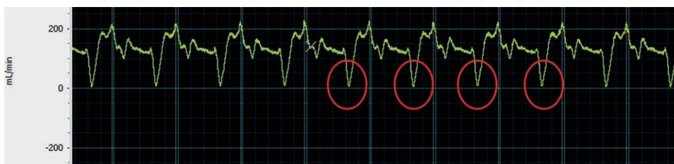
Figure 3. Coronary flow in ml/min curves obtained with the circuit (LabChart 8 pro screenshot). Circled in red, the drop in flow during systole, obtained by extrinsic compression of the coronary model in synchrony with the pump.
