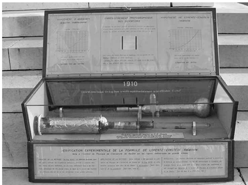
Fig. 9. The wooden casket containing the two cathode-ray tubes that Guye used in his experiments. The lower one was used in his second, decisive experiment. Credit: Museum of History of Science, Geneva.
