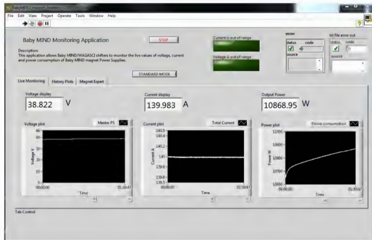
Figure 5-17: LabView program for live monitoring of the magnet power supplies.
