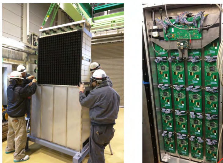
Figure 2-23: Wagasci module installation into the water tank (left). Electronic readout cards based on SPIROC chip.
