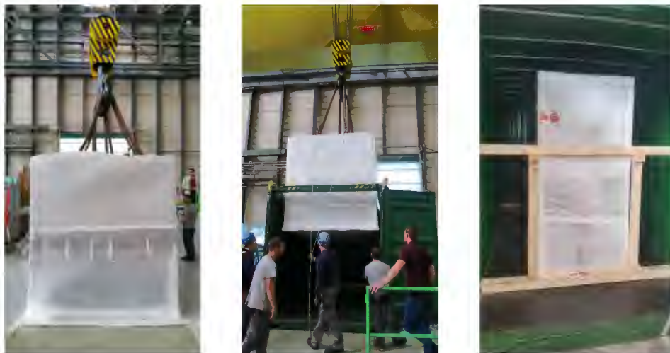
Figure 5-3: Loading detector chassis into the transport containers.
