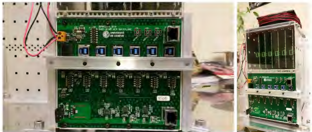
Figure 3-90: The 6 FEBs in a mini crate are daisy chained together via the back plane.
