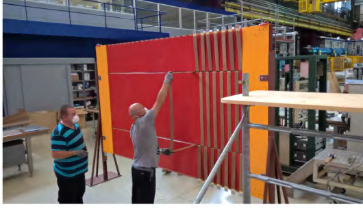
(c) Insertion of U shaped Aluminum conductor
