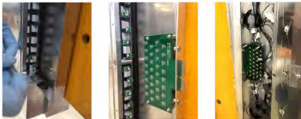
Figure 3-41: Assembly of MPPCs onto the scintillating modules.
