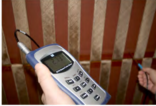
Figure 3-18: Hall probe on the surface of magnet module measures 2.7 mT, confirming that there is not significant flux leakage.
