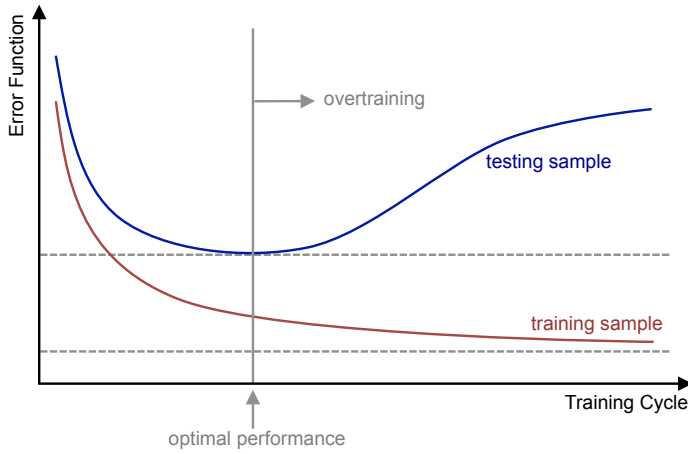
Figure 6.2: Example of the error function development for an over-trained network. The red (blue) line shows the development of the error function evaluated on the training (testing) sample over the course of the training epochs. When training beyond the point of the optimal performance marked by the vertical gray line, the error function continues decreasing for the training sample, while it starts increasing for the testing sample.
