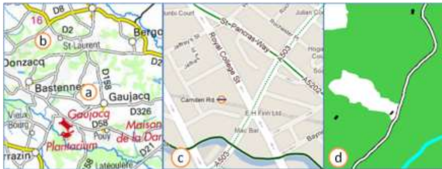
Fig. 1 The town symbol is on the road when it actually crosses the town (a) or near the road when it passes by the town (b) (©IGN). (c) The relation “the cycle path follows the road” facilitates the symbolising of the road with the dotted line. (d) The relation “the building is inside a clearing” should be preserved by generalisation.
