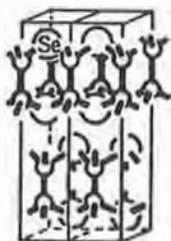
Figure II - 6 : Crystal structure of \epsilon - GaSe 2H, hP8 and its crystal chemical formula in two versions.
