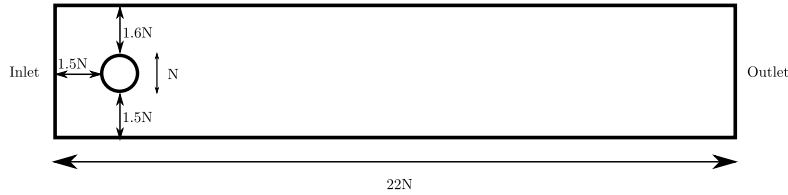
Figure 13: Geometry for the flow past a cylinder.
