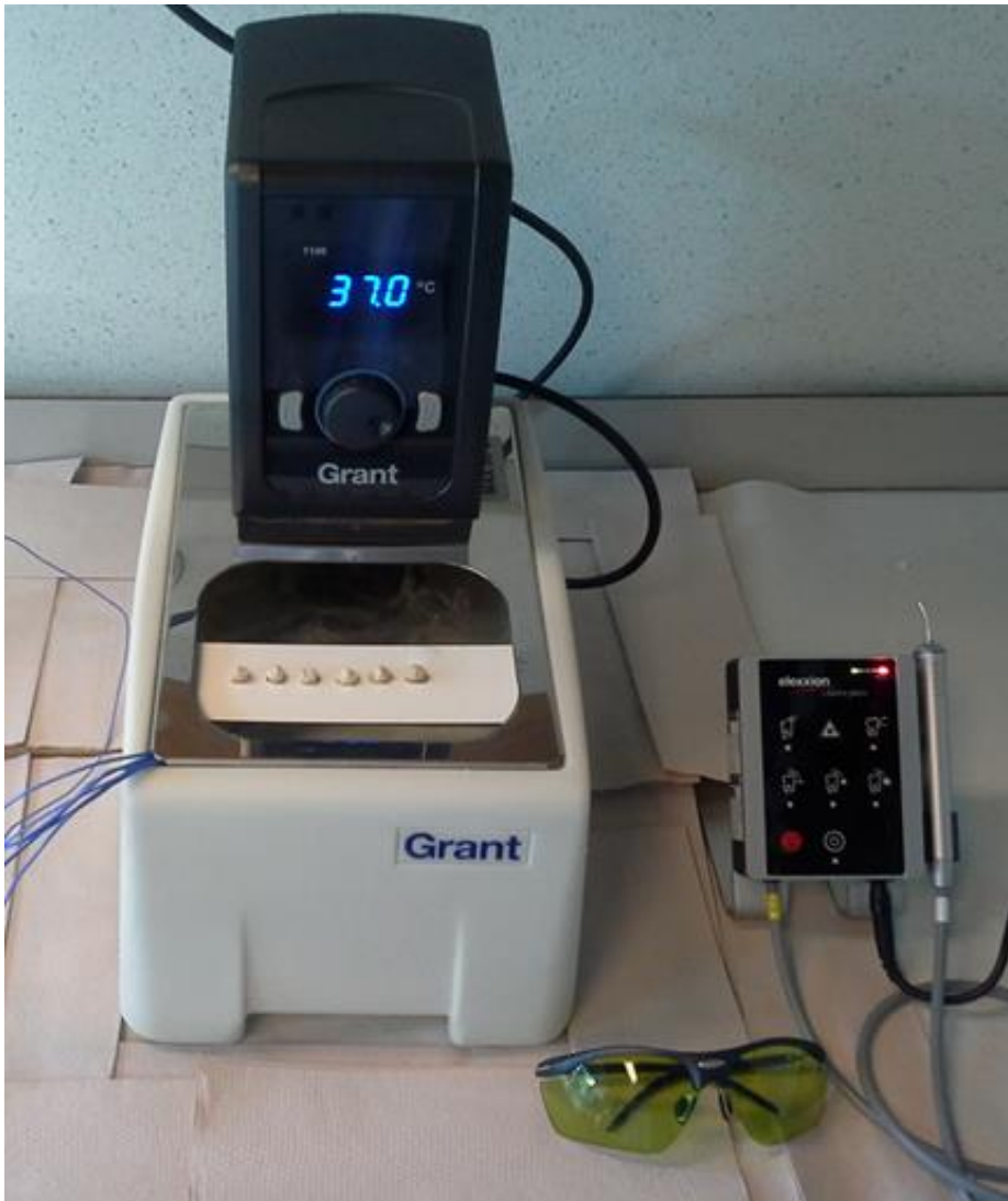
FIGURE 1 : Teeth samples mounted on a platform and immersed in 37°C water bath
