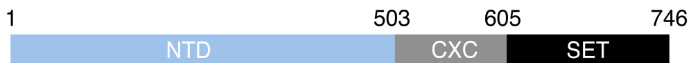
Figure 10. EZH2 structure. Boxes identify the main domain of EZH2: the cysteine-rich CXC domain; the catalytic SET domain; and the N-terminal domain (NTD) which provides binding sites for several interactors.
