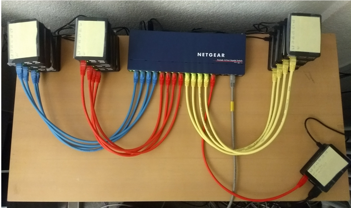
Figure 5.5: A Spark cluster of 13 Raspberry Pis. Master node (bottom right) and worker nodes connected via an ethernet switch.
