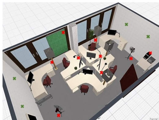
Figure 3.4: 3D representation of office environment. Green marks are sensors and red marks are actuators.
