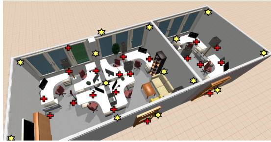
Figure 6.2 – Office Environment of implementation. The cross represents the electrical-electronic interface and the "star" the sensors for monitoring the environment
