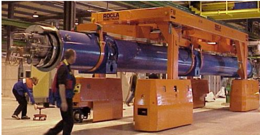
Figure 3.2: The ROCLA, the special vehicle design for the transportation of the LHC superconducting dipole magnet.
