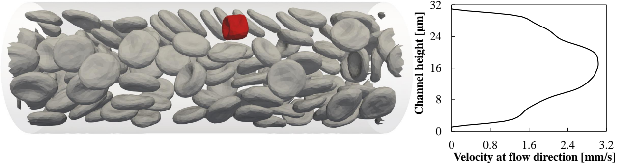
Figure 9: Simulated Poiseuille flow with no interpenetrations. The marked red blood cell (in red) has developed a multilobe shape as described in Lanotte et al. 2016 [70]. The graph shows a temporal average of the velocity at the flow direction in the middle of the tube.
