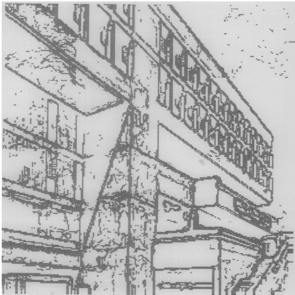
FIG. 12. Picture obtained by thresholding blocks of 64 \times 64 pels (from Fig. 7a).
