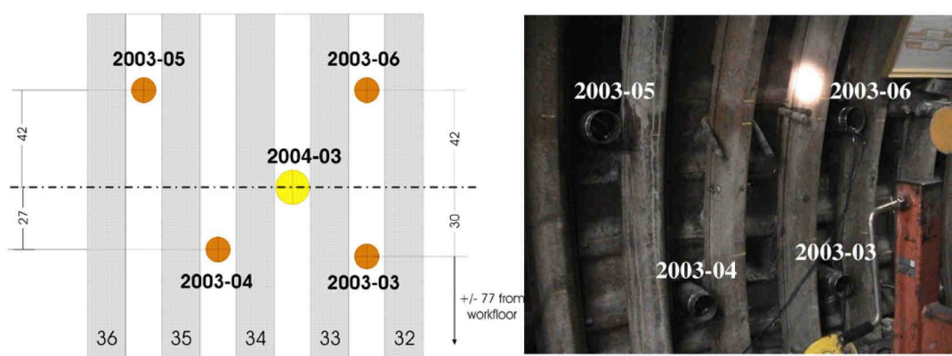
Figure 3-45. SELFRAC-IV collapsing borehole experiment Location map (left) and photograph (right) of the four observation boreholes and the central collapsing borehole
