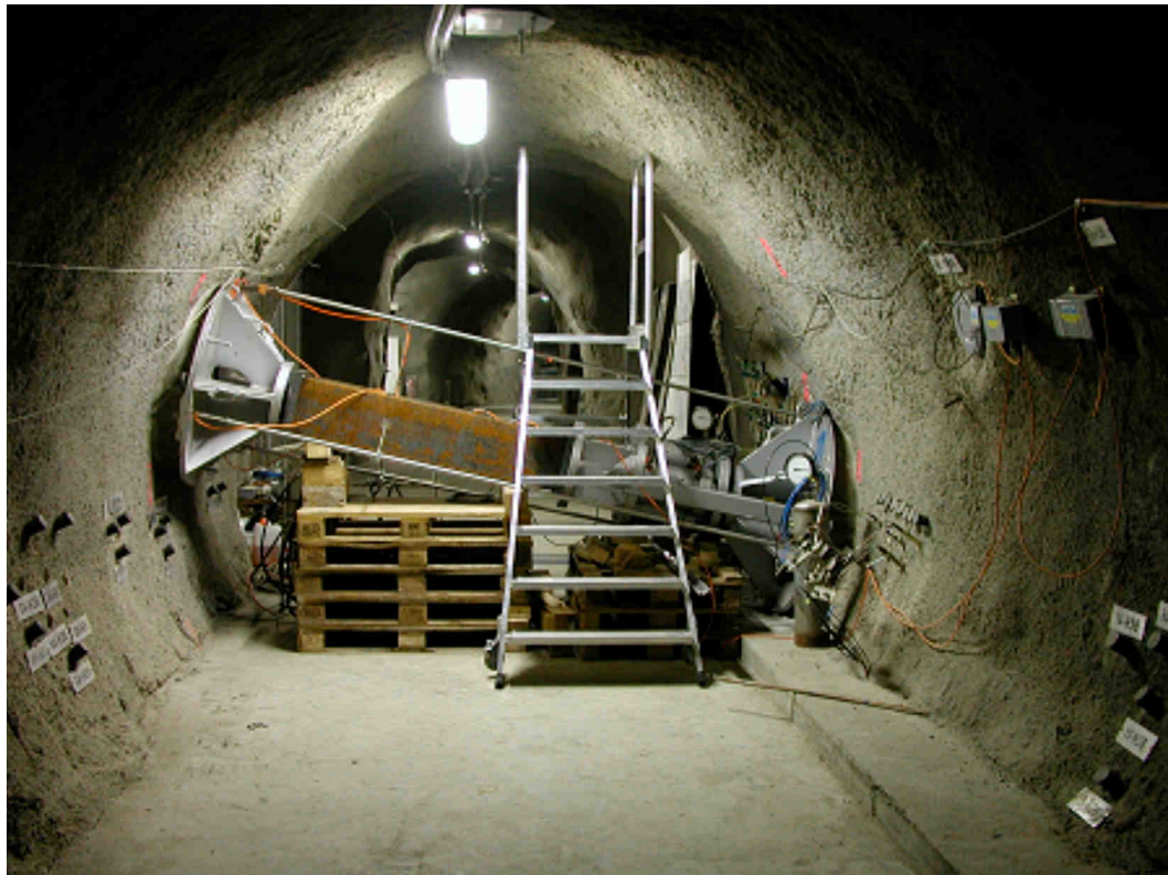
Figure 3-31. SELFRAC-I plate load testing set-up in the Gallery 98 of the Mont Terri URL (from Heitz et al. 2003)
