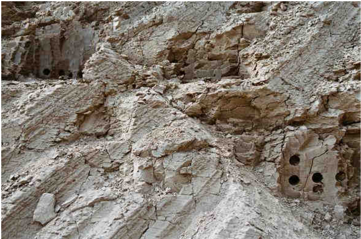
Figure A.4-2. Normal fault in the Boom Clay at Kruibeke, Belgium, with a throw of some 50 cm Note core sampling holes in the hanging wall (bottom right) and footwall (top left) of the fault plane for investigation on the structural and mechanical changes adjacent to the fault plane (from Dehandschutter et al. 2005b)
