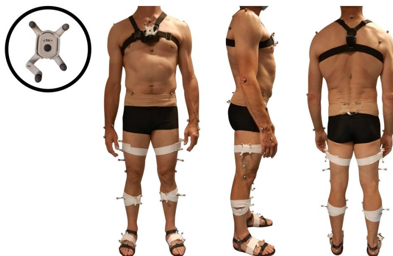
Figure 1. Equipment including 7 inertial sensors (Physilog6S, GaitUp) and reflective markers on the clusters and body landmarks (Conventional Gait Model 1.0).
