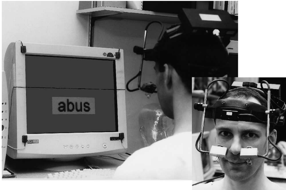
Fig. 1. The SMI EyeLink system. Three cameras are attached to a headband. Two cameras are recording eye movements. One camera is recording IR light points from each corner of the screen to monitor head position relative to the screen. On this basis, the EyeLink software calculates online the gaze position in screen coordinates. In this example, a 4-letter word is projected on a stabilised retinal area located at 5° eccentricity in the lower visual field. The horizontal line crossing the screen represents a fixation aid for the subject (used in experiment 1).
