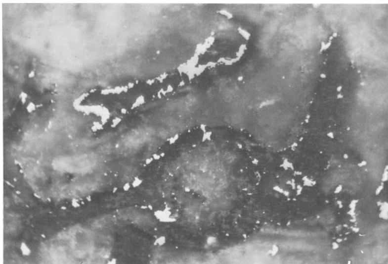
Fig. 7. Glassshards in unwelded tuff (unit B2) replaced by quartz, chalcocite, and bornite. Photo length: 0.33 mm. Polished section, uncrossed nicols
