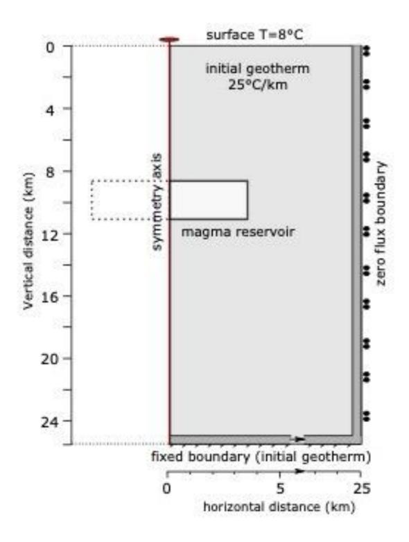
Figure S1: Geometry of the axisymmetric thermal model. Instantaneous intrusion of a cylindrical magma reservoir at 10 km depth is modelled for magma volumes of 100, 1000 and 10.000 km³. The surface temperature is fixed at 8°C and the initial geothermal gradient is set to 25°C/km. Upper and lower boundaries are fixed temperature, while a zero flux condition is imposed on the right boundary. The left boundary of the model is the plane of symmetry.
