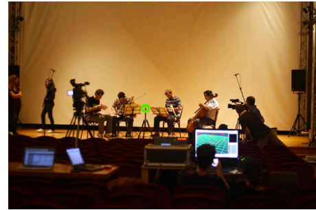
FIGURE 1 | The multimodal setup for the experiment, showing motion capture, videocameras, and environmental microphones. Each musician wears markers for motion capture. Piezoelectric microphones are in the body of the instrument. Note the position of the SQ ear represented by the optical reflector placed on the tripod situated in the center of the quartet, equidistant from the four musicians.
