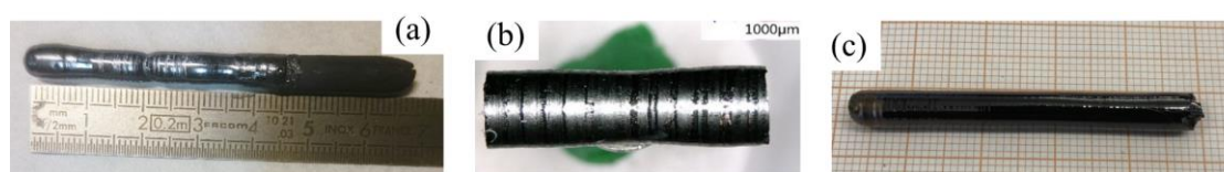
Figure 4.4 | Photographs of as-grown single crystals with floating zone technique. As synthesized single crystals of (a) and (b) Nd_2NiO_{4.23} and (c) Nd_{1.5}Sr_{0.5}NiO_{4.05} .
