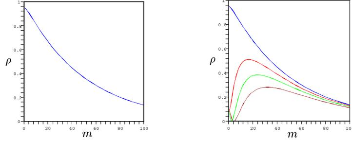
**Fig. 2.** **Left:** Behavior of the convergence factor  $\rho_{cla}$ . **Right:** Comparison between  $\rho_{cla}$  (top curve),  $\rho_{T0}$  ( $2^{nd}$  curve),  $\rho_{T2}$  ( $3^{th}$  curve) and  $\rho_{O0}$  (bottom curve). In both plots  $a = \pi - L/2$  and the overlap is  $L = b - a = \frac{1}{100}$  and  $\eta = 2$ .
