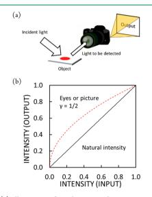
**Figure 1.** (a) Illustration of a colorimetric detection system where a picture is taken and output on a screen and (b) relationship between input and output light intensity in the absence (black line) and presence (dashed line) of gamma correction.
