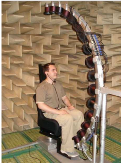
Figure 2-18. Taken from [69]. Equipment for fast personalized HRTF measurements. The speakers located on the arc produce wide spectrum sounds recorded by microphones placed in the ear canals. The chair rotates automatically, powered by a step motor, allowing for fast collection of HRTF data from all directions around the listener.
