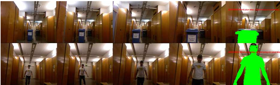
Figure 3-67. Two sequences in which the alerting system has detected an entity potentially leading to a stumble (or collision). First row, the users moves toward an unexpected obstacle (serendipitous encounter). Second row, the obstacle (a person) rushes over the user (threatening approaching). Once detected, the system segments the object and launches a warning message in either case.
