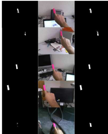
Figure 3-55. The segmentation of a pinkish marker stuck on a fingertip. The central column shows the original color images provided by the camera. The left column present the binary segmentations achieved over the RGB color space. In turn, the right column show the segmentations achieved over the Lab color space. Out of this example and experimental observations made in this work, it becomes clear that the segmentation on Lab color space turns out to be more robust.
