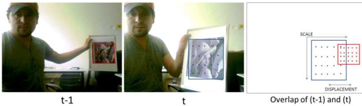
Figure 3-57. Tracking of an object (a picture of Lena) using the Kalman Filter. The KF maps the sampled points ( \mathbf{y}_{t-1} ) of an object (in one frame t-1 ) into \mathbf{y}_t (the same points of the object in the frame t ). It results in a sparse motion field (the dispersion of the points in the 2-dimension space). Based on this motion field, the scale and the displacement ( \mathbf{x}_t ) of the object bounding box in the frame ( t ) can be calculated with respect to \mathbf{x}_{t-1} .
