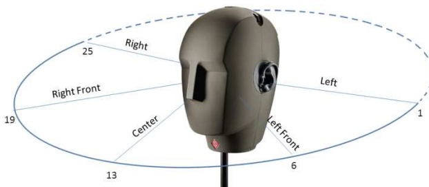
Figure 3-8. Spatialization of sound in See CoOr. Sounds can be perceived as approaching from 25 different positions (from right to left) across the azimuth-frontal auditory field.
