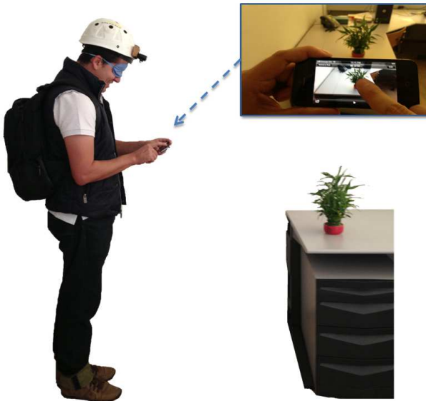
Figure 3-51. A user interacting with our global module based on a tactile interface. A zoom into his hands is shown top-right of this image to clearer see how the interaction takes place on the iPhone screen.
