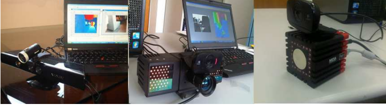
Figure 3-26. Three mounted systems, from left to right: (RGB-Kinect) HDWebcam-KinectMicrosoft, (RGB-CamCube) HDWebcam-PMDCamCube, (RGB-SR4000) HDWebcam-SwissrangeSR4000.
