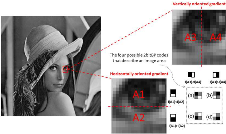
Figure 3-58. Here we present the four possible 2bitBP codes (a, b, c, d) that describe the surrounding area of a point in the image (around the eye). In 2bitBP approaches the scale and aspect ratio of this area are usually generated randomly (though rather small). Within this area four subareas can be extracted (A1, A2, A3, A4) when viewed horizontally and vertically. The final 2bitBP code is made out of the comparisons between vertical and horizontal subareas. The comparison is based on which subarea has a major integral value I (the sum of its pixels). Given that, in this particular example, I(A1) > I(A2) and I(A3) < I(A4) , the 2bitBP that describes the area is (c) (i.e. [01 11 00 01], with 00=gray, 11=white, and 00=black).
