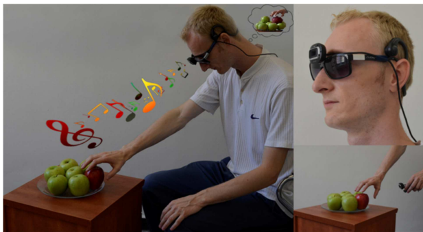
Figure 2-43. (taken from [33]) Left: An illustration of the EyeMusic sensory-substitution device (SSD), showing a user with a camera mounted on his glasses, and using bone-conductance headphones, hearing musical notes that create a mental image of the visual scene in front of him. He is reaching for the red apple in a pile of green ones. Top right: close-up of the glasses-mounted camera and headphones; bottom right: hand-held camera pointed at the object of interest.
