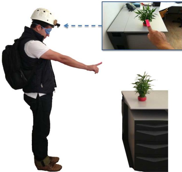
Figure 3-52. A user interacting with our handsfree version of the global module. On top-right of this figure, we display also the image captured by the head-mounted camera. Such image contains the user fingertip that has been enhanced with a marker.
