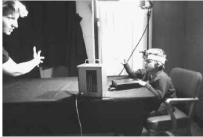
Figure 2-25. (taken from [34]) Using the Optacon the child in this image was able to mimic the hand posture of the teacher using feedback acquired via the device. The first prototype was completed on 1969. It was portable and combined the stimulator array, electronics, batteries, and camera in a single package measuring 13.5" by 8" by 2.25". The total weight of this device was 9 pounds.
