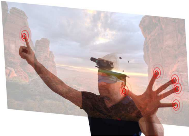
Figure 3-31. Tactile-sound interfaces would allow unsighted individuals accessing information of an image via touch. The idea underlying here is that a user can hear elements of the real world by pointing (or touching) them with the fingers, as shown in this figure. Ideally, the user needs only to sweep (explore) the real world with his hands and fingers in order to get visual information. In an attempt to reproduce this idea, in See CoLoR we capture the appearance of the real world into an image that is presented to the user through a tactile tablet. Thus, instead of naturally pointing into the real world, See CoLoR's users need to carry a tablet and point (tap) into it in order to explore the sonified visual information. The implementation of this tablet-based interface will be discussed in this section, whereas seminal ideas and early implementations of the ideal model (tablet-free) will be exhibited later in the conclusion section of this work.
