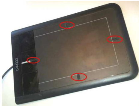
Figure 3-36. Touch pad on which grid images are represented during the game. The circles highlight the four markers indicating the middle of the edges of the sensitive area.
