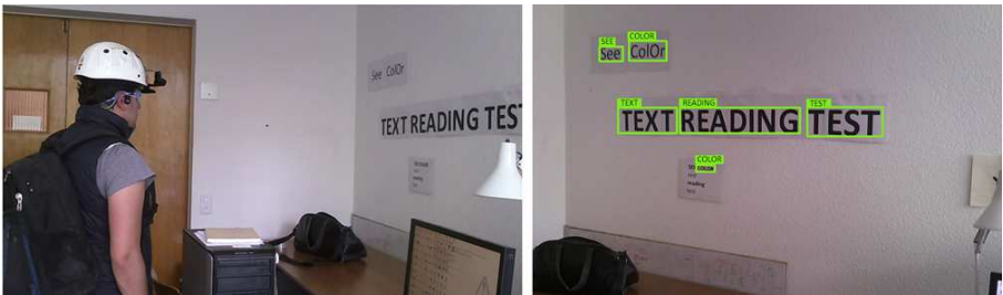
Figure 3-72. For this experiment the TRitW was retrained using simple Calibri-font characters with white background. Also, we used a lexicon consisting in five words: {COLOR, READING, TEST, TEXT, SEE}. Finally, we use the function TTS (text-to-speech) in matlab to translate the results of TRitW into voice. In the left image there is a See CoLoR user scanning the wall. Note that an external color camera has been coupled to the Kinect sensor.
