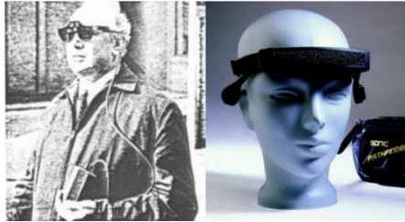
Figure 2-32. The evolution of so-called sonic pathfinders from the 60's (left [89]) up to 2012 (right). In the 80's there was a proliferation of research and production of such devices.
