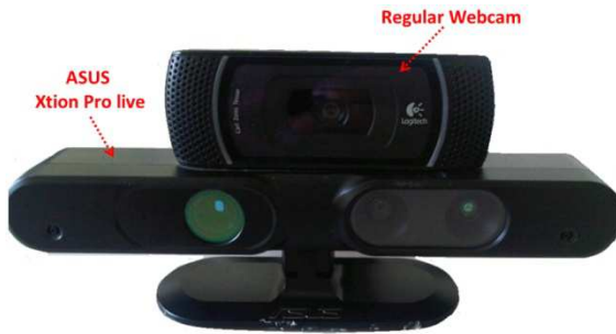
Figure 3-3. Coupling of a 3D sensor (ASUS Xtion Pro Live) with an external camera (regular webcam) to increase color resolution for better performance in computer vision applications.
