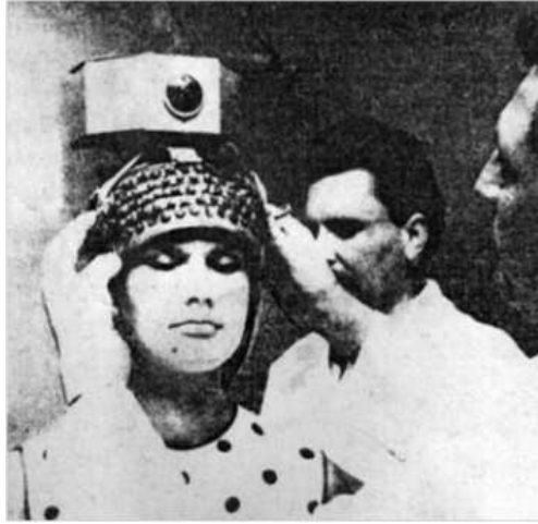
Figure 2-19. (taken from [73]) Later version of Noiszewski's Elektroftalm (1970).
