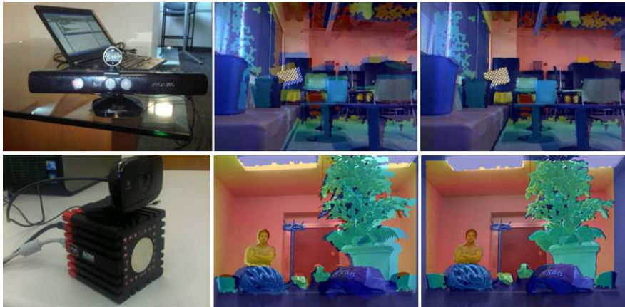
Figure 3-18. Coupling of color and range cameras: Leftmost column shows two mounted systems made up by depth sensors (Kinect on top, SwissRanger SR-400 at the bottom) and a HD web camera. In the middle column the re-sized depth maps and the color images (webcam) have been merged. In the rightmost column finally, we repeat the merging right after the depth maps have been registered into the color images using our algorithm. A twofold aim may be targeted: the addition of depth in a HD cam or the improvement in color resolution of kinect. Moreover, images at the bottom of this figure may attest that our algorithm is valid for complex scenes which exhibit flexural 11 geometry.
