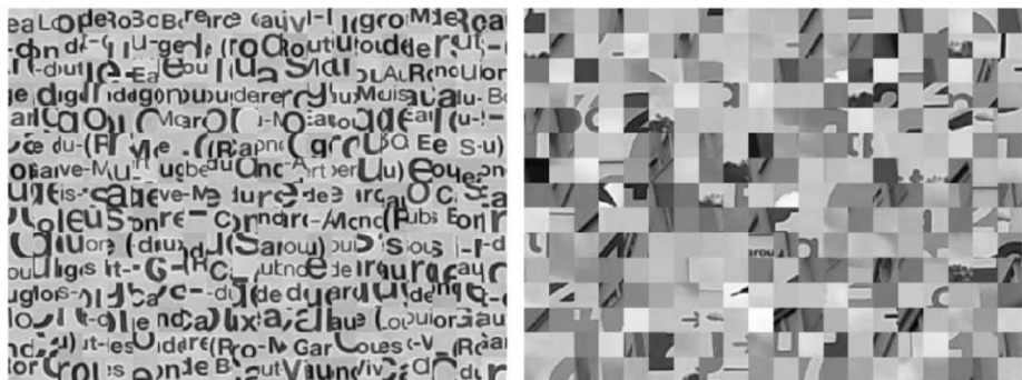
Figure 3-78. Classes: “text” or positive (left) and “not text” or negative (right). In this figure 300 examples (20x20 pixels each) of each class are shown, the whole amount of positive and negative examples serves as a training data set for our binary network (detector).
