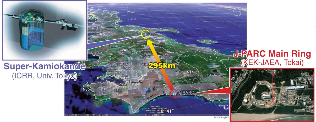
Figure 3.1: Overview of the T2K experiment, where a high intensity beam of \nu_\mu is created at Tokai and sent 295 km under ground to Super-Kamiokande.
