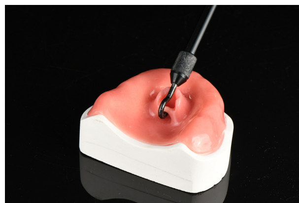
Figure 2. Retention testing platform with dynamometer hook.
