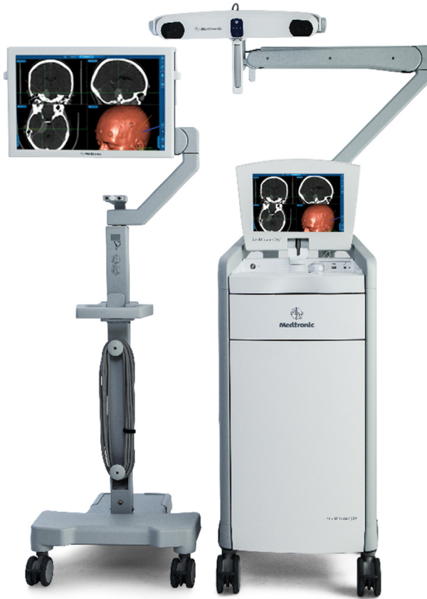
Fig. 4. Medtronic's S7 StealthStation. The S7 is the most recent model of Medtronic's image-guided surgery platform. On the left is a large high-definition touch-screen monitor. To the right is the navigation computer and planning workstation. Note that the infrared camera used for optical tracking is attached to the workstation and positioned above the surgical field.
