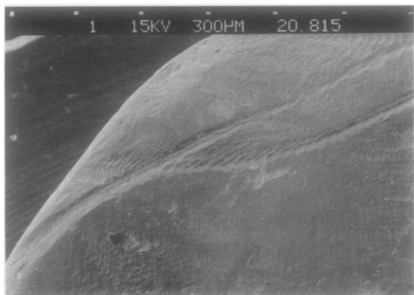
Fig. 3. Scanning electron microscopic view of surface of sample after removal of residual composite. Note grooves and scratches caused by tungsten-carbide bur.
