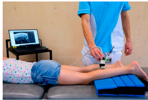
Figure 5. Illustration of the ultrasound set-up, including the motion tracking system (OptiTrack) and the B-mode ultrasound unit with a linear transducer (Telemed Echoblaster), both connected to a laptop for synchronized image and motion data acquisition and real-time display.
