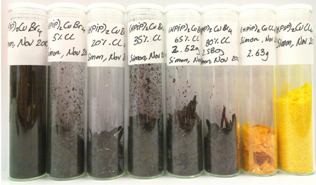
Figure 2. Complete Br/Cl substitution series (\text{Hpip})_2\text{CuBr}_{4(1-x)}\text{Cl}_{4x} , x=0 (left, black) and x=1 (right, yellow).
