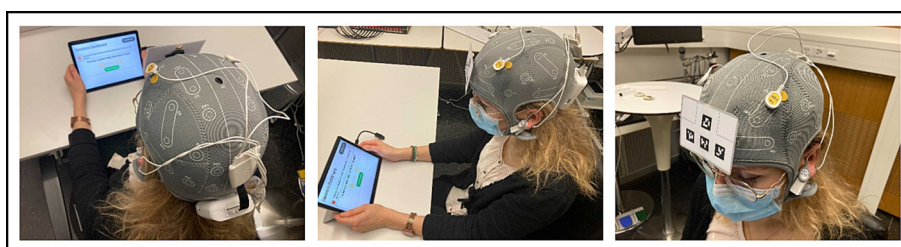
Fig. 2. CURRENT complete set-up. Depicted including neoprene cap, tablet and tDCS device (Starstim-Home Neuroelectronics), as well as QR-like markers for cap placement evaluation.
