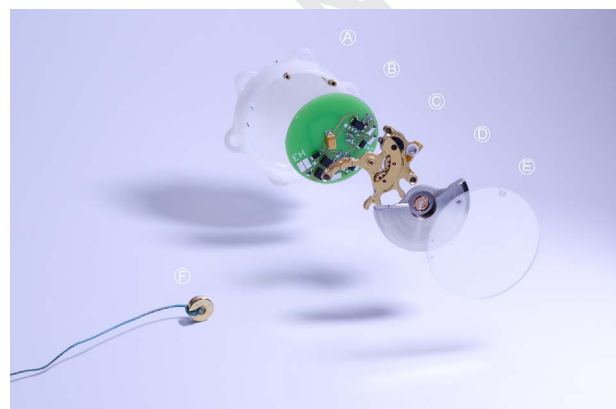
Figure 4 Disassembled lead- and batteryless pacemaker: Explosion view of the pacemaker depicting (A) housing with pacemaker electrodes and jacks for lead measurement and 2 metal inhibition pins, (B) pacemaker circuit, (C) skeletonized clockwork, (D) oscillation weight, (E) transparent lid, and (F) permanent magnet to inhibit pacing.
