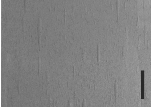
Figure 3. Sheared bubbles visible at the pipe walls during a syrup-air experiment ( u_{sg} = 0.06 m/s). Scale bar is 2 cm long.
