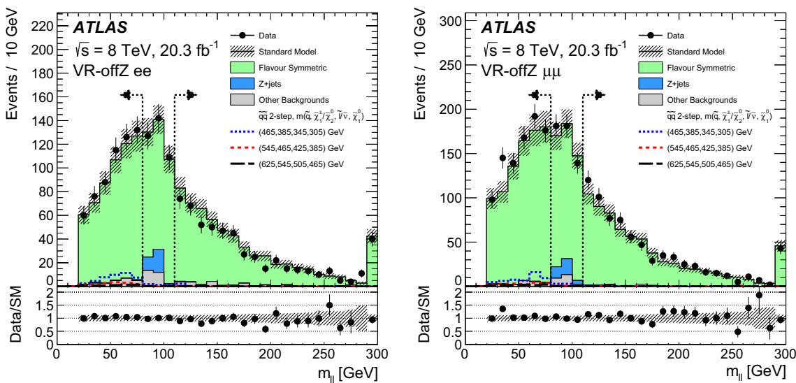
**Fig. 5** (Corrected version): The observed and expected dilepton mass distributions in the electron (*left*) and muon (*right*) channel of the validation region (VR-offZ) of the off-Z search. Data (*black points*) are compared to the sum of expected backgrounds (*solid histograms*). The *vertical dashed lines* indicate the  $80 < m_{\ell\ell} < 110$  GeV region, which is used to normalise the  $Z + \text{jets}$  background. Example signal models
