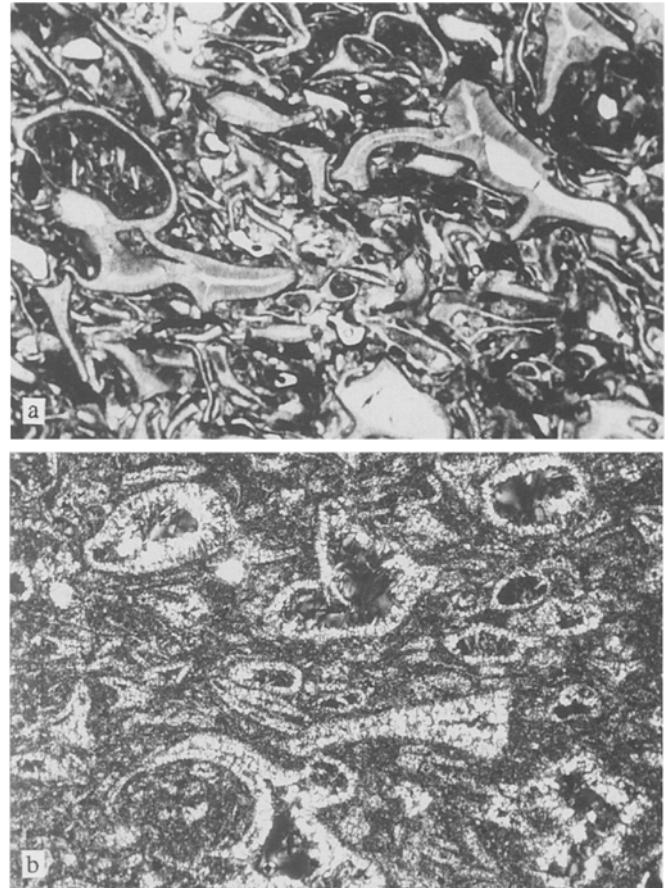
Fig. 10 a Cryptocrystalline vapor phase facies. Vitroclastic texture is retained despite 100% devitrification into very fine elongated crystals forming axiolitic structures, under plane light; white areas are vesicles. Silica phase is cristobalite. Horizontal field of view is ca. 3 mm. b Microcrystalline vapor phase facies. Same scale as above with crossed nicols, poorly developed vitroclastic texture seen only under microscope due to coarseness of more granular crystals. Note vesicles (black ovals) lined with largest crystals. Silica phase is mainly tridymite
